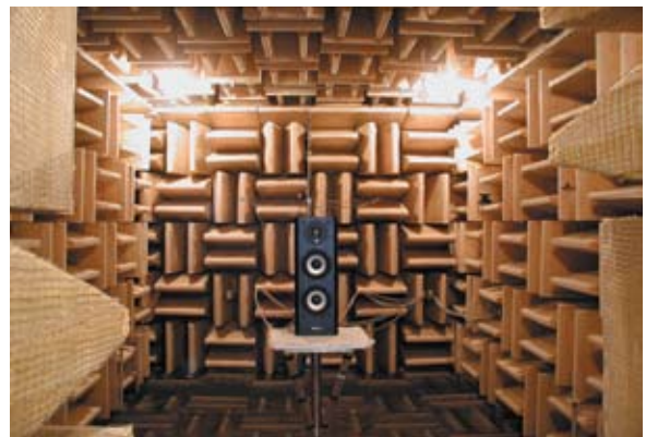
The M22 v2 being tested in the anechoic chamber at the National Research Council.
